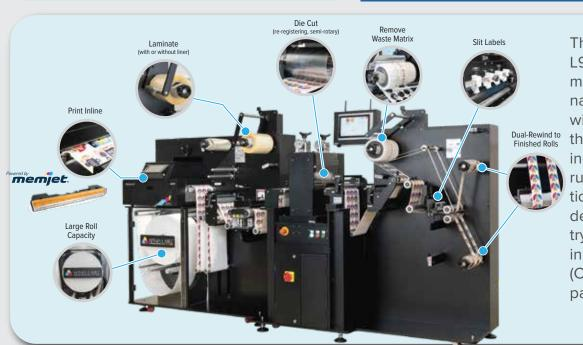
The integrated L901's printer makes maintenance possible with the media threaded, allowing for uninterrupted production. In addition, it delivers industry-leading low ink costs via five (CMYKK) high-capacity cartridges.
